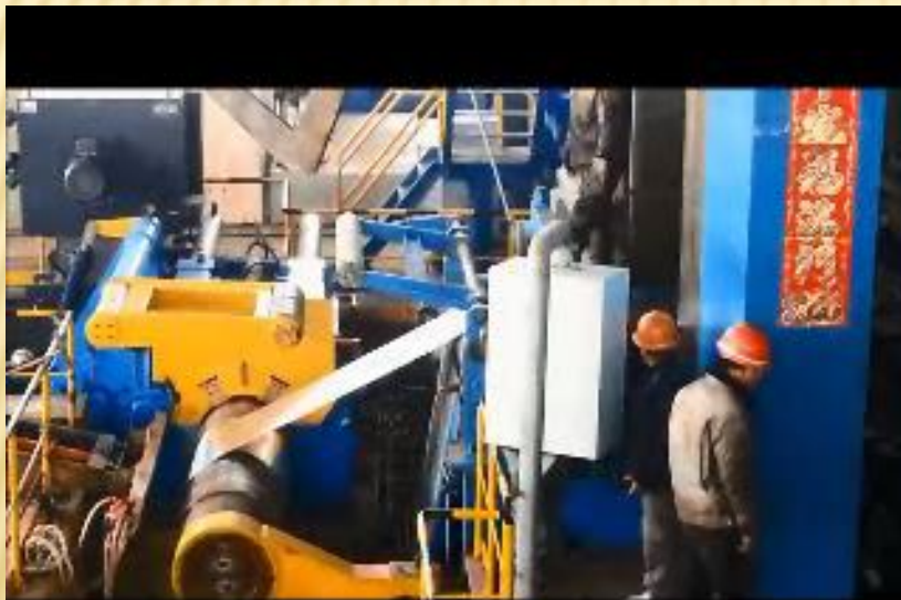
Magnesium strip rolling line
