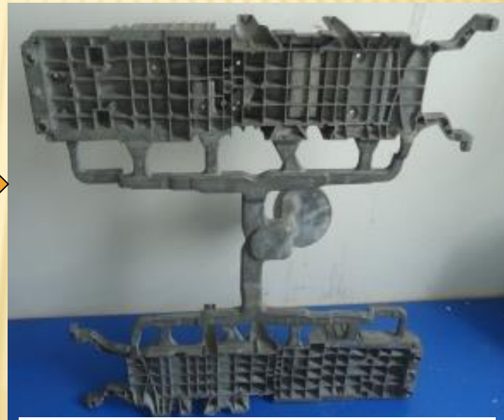
Casting: One mold two pieces
