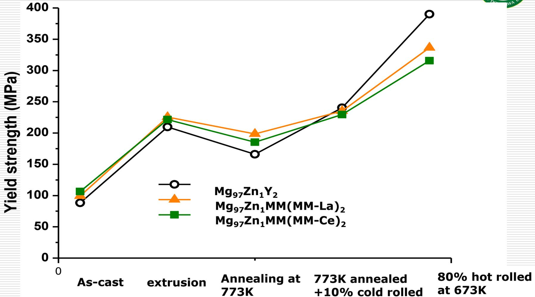
The extrusion improves the yield strength, annealing declines the strength due to the recrystallization, and cold or hot rolling can increase the yield strength because the particle size of second phase was refined.
