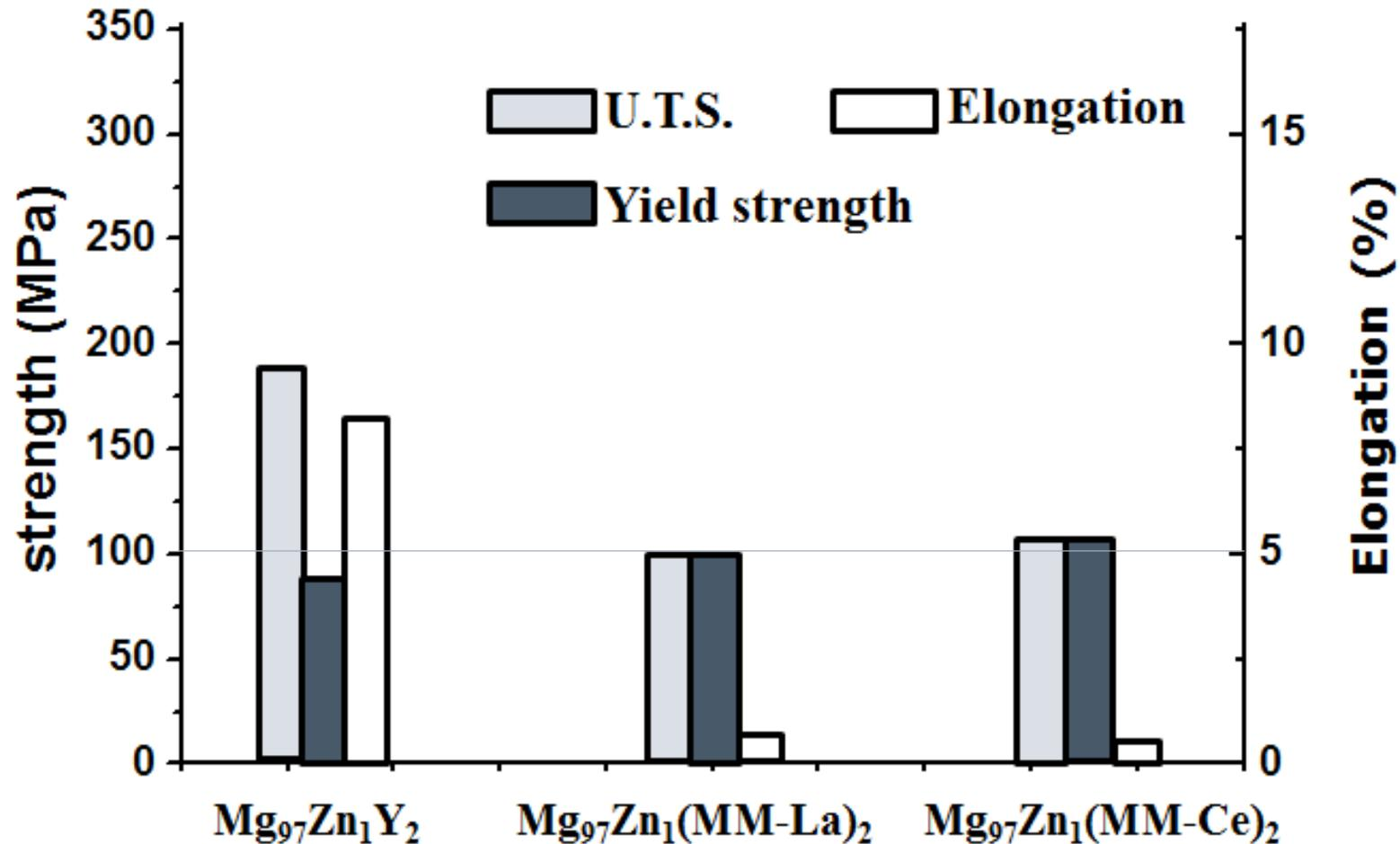
The yield strengths of both  $Mg_{97}Zn_1MM_2$  alloys are higher than that of  $MgZnY_2$  alloy.
