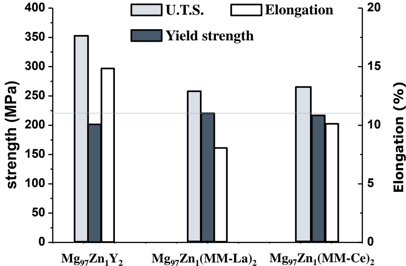
The yield strengths of all alloys are improved due to the contribution of fine structure. And strengths are increasing by almost two times comparing with as-cast ones.
