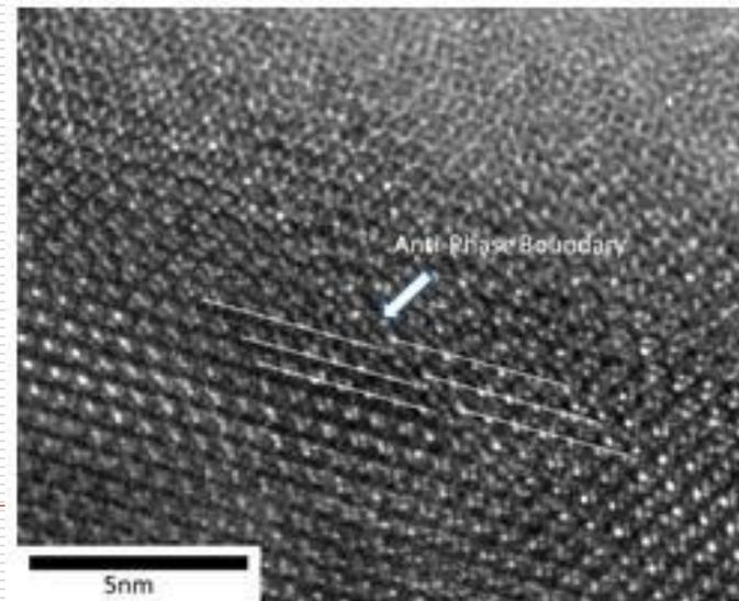
(a) HR-TEM lattice image and diffraction pattern, and (b) HRTEM image of interface between  $(\text{Mg, Zn})_{12}(\text{La, Ce})$  and matrix.
