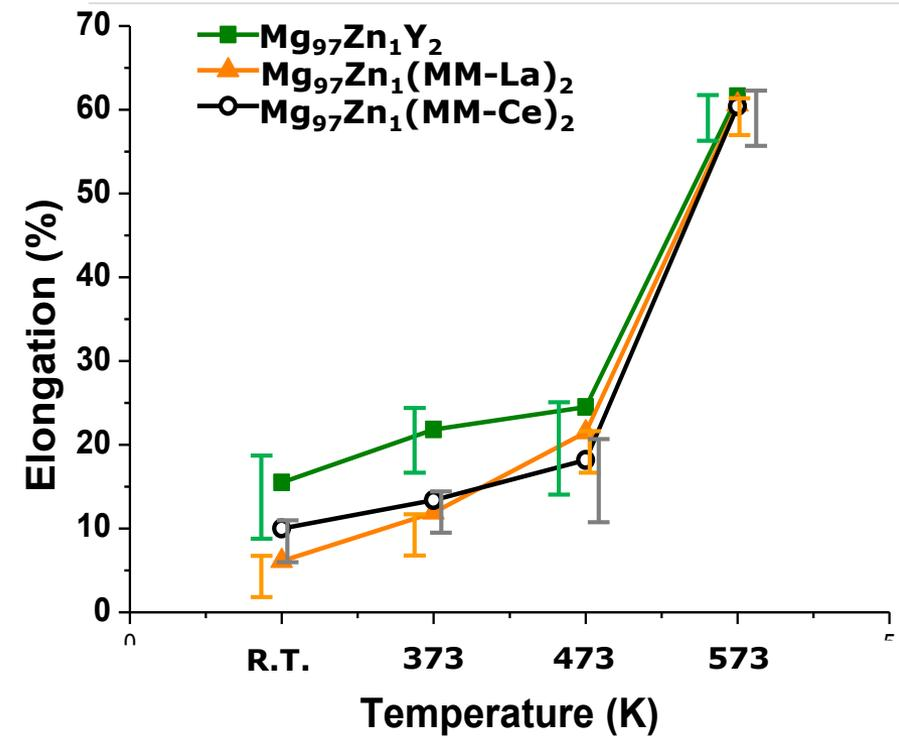
The high temperature mechanical properties of both  $Mg_{97}Zn_1MM_2$  alloys are a slightly worse than that of  $Mg_{97}Zn_1Y_2$ . That means the LPSO phase have a stronger heat resistance than that of second phase in  $Mg_{97}Zn_1MM_2$  alloys.
