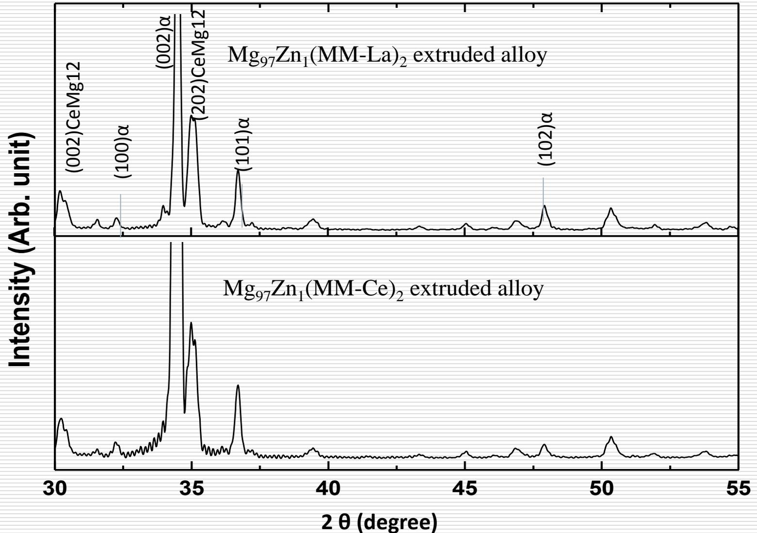
The second phase in both  $\text{Mg}_{97}\text{Zn}_1\text{MM}_2$  alloys is confirmed as  $(\text{Mg,Zn})_{12}(\text{La,Ce})$ .
