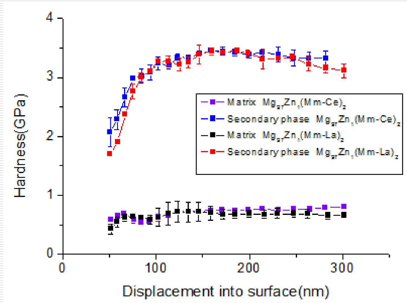
The hardness of second phase in  $Mg_{97}Zn_1MM_2$  alloys is about 5 times higher than that of matrix.
