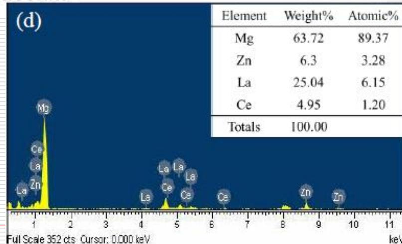
(a) TEM image, (b) SADP of particle, (c) SADP of matrix, and (d) EDS result of particle.
