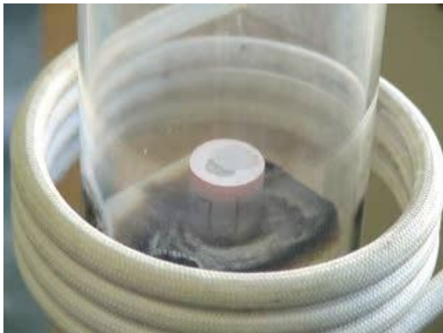
Combustion foaming behavior
