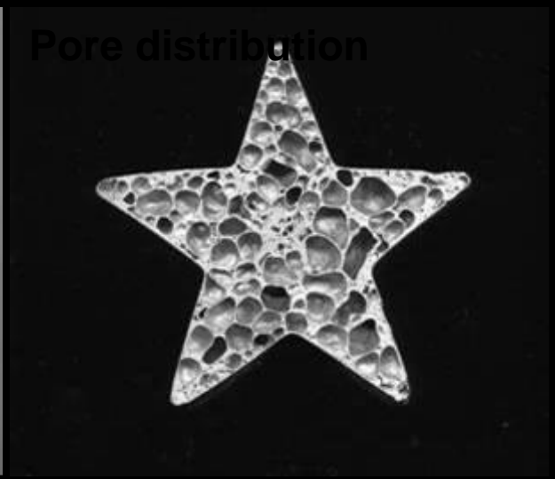
Porous Al filled in a hollow tube
