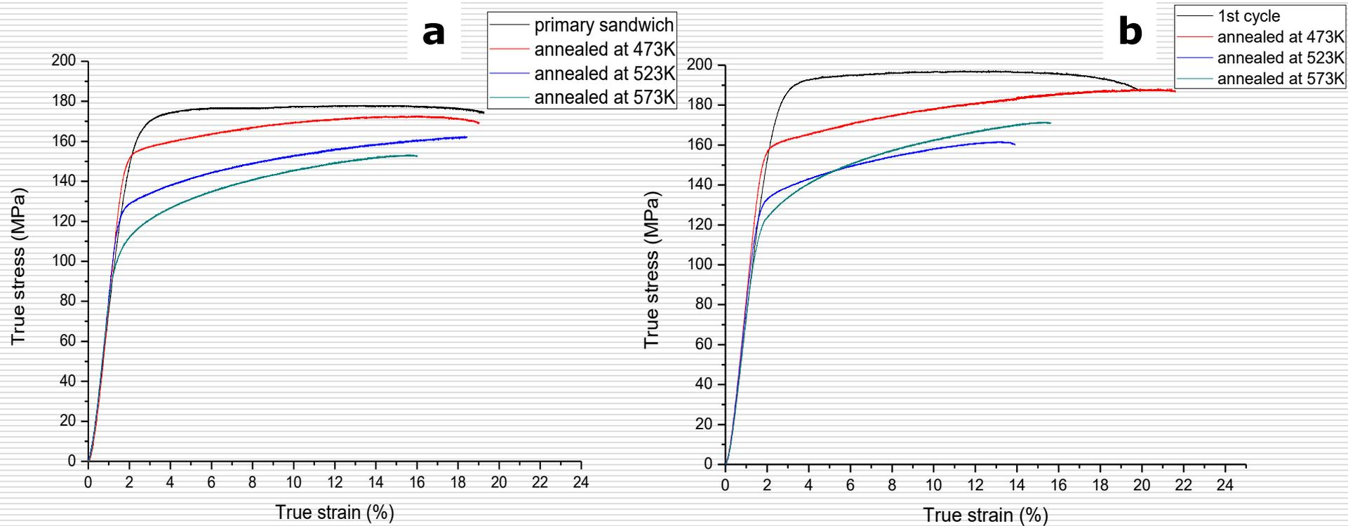
True stress-strain curves of (a) primary sandwich and (b) 1 cycle ARBed Al/LZ91/Al multilayers after annealing at different temperature.
