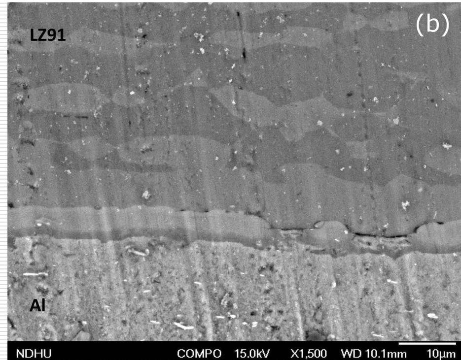
SEM cross-section images of 1 cycle ARBed Al/LZ91/Al after annealing at (a) 473K, (b) 573K.
