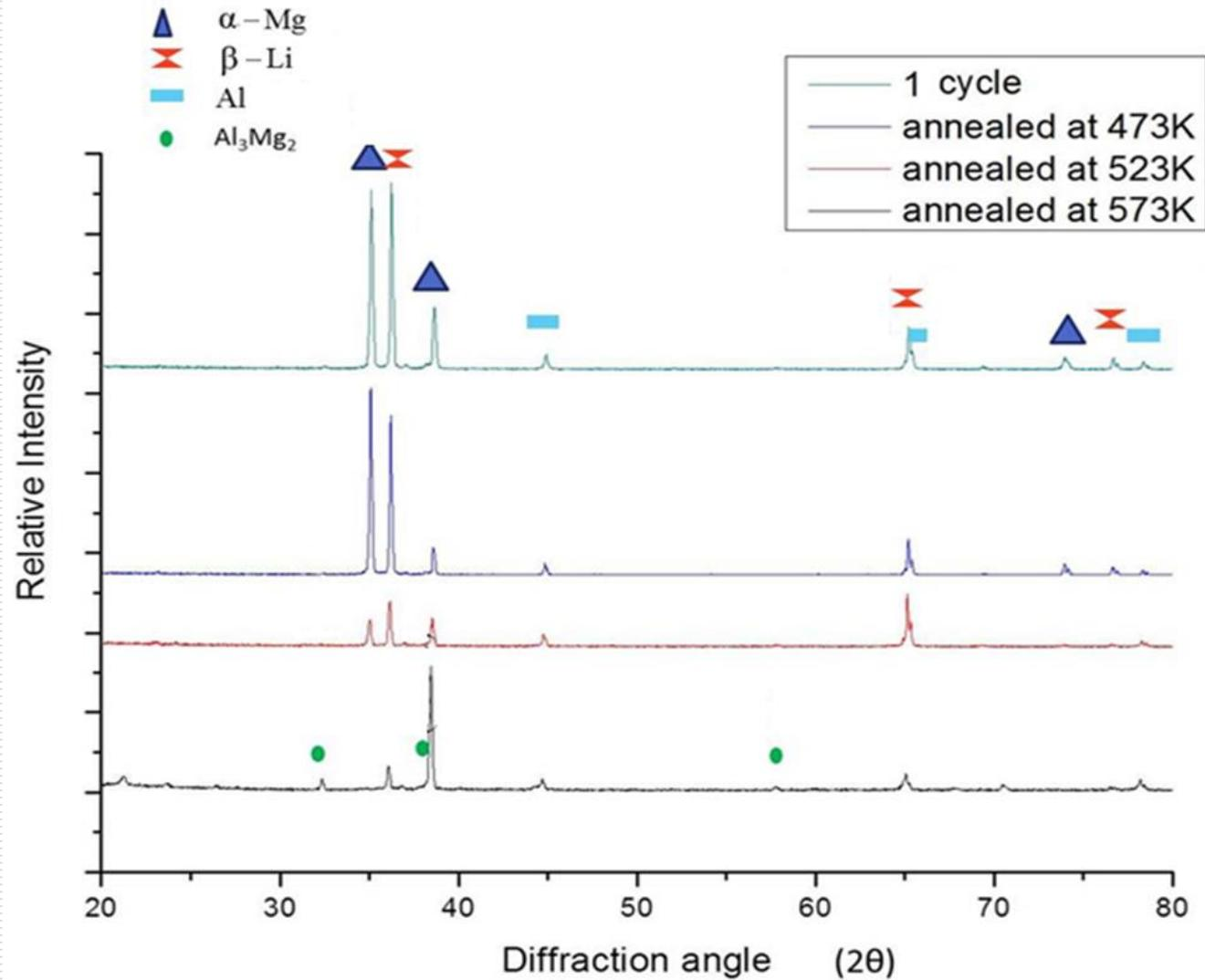
XRD spectrums of 1 cycle ARBed Al/LZ91/Al after annealing at (a) 473K, (b) 523K and (c) 573K.
