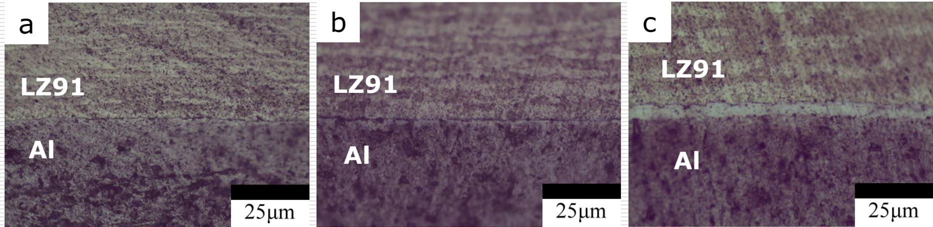
Cross-section optical micrographs of Al/LZ91/Al **primary sandwich** after annealing at (a) 473K, (b) 523K and (c) 573K.
