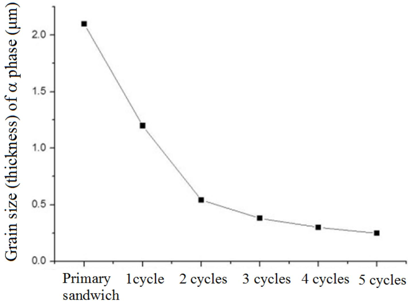
The grain size of  $\alpha$  phase in LZ91 side of composite after different number of ARB cycles
