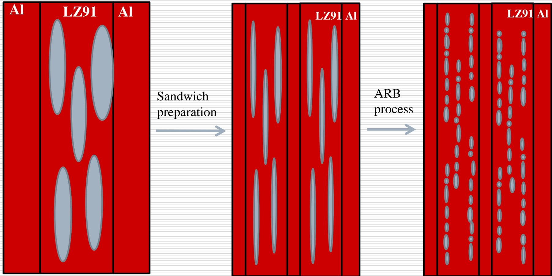
The size of  $\alpha$  phase in LZ91 was thinned after primary sandwich and broken down to small particles after ARB process. Therefore, the grain refining and strain hardening of both materials increased the strengths of multilayered Al/LZ91/Al.
