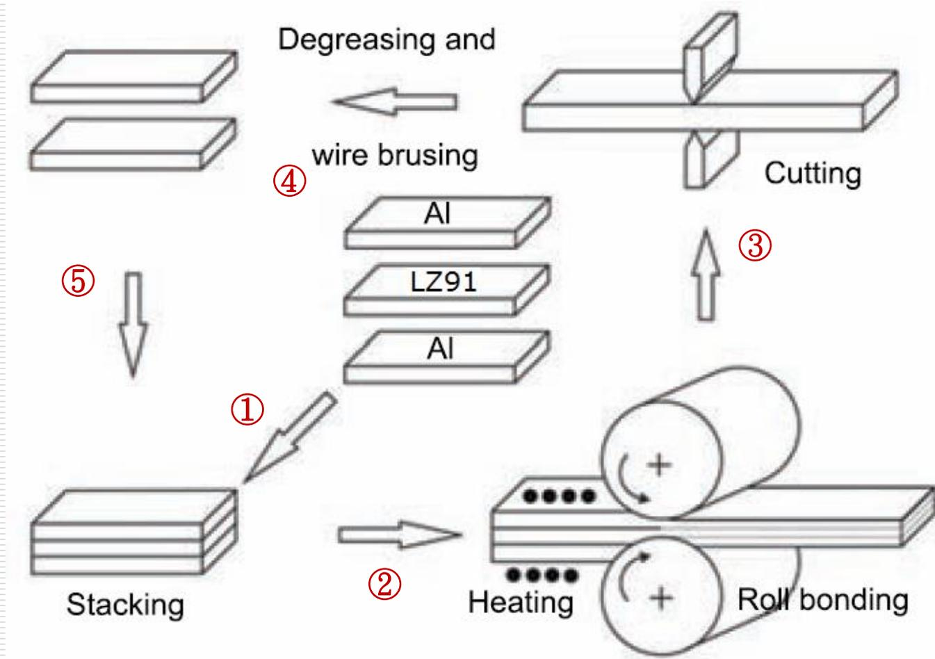
First, the Al and LZ91 sheet surfaces were cleaned and stacked together. The stacked sheets were kept in a furnace and then hot roll-bonded. Then the roll-bonded sheet was cut into two parts with the same dimensions. After the surface cleaning, the two parts were stacked together ready for another ARB.
