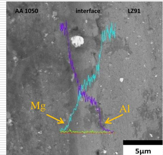
BSE images and EDS line scan of 1 cycle ARBed Al/LZ91/Al after annealing at (a) 473K, (b) 523K and (c) 573K.
