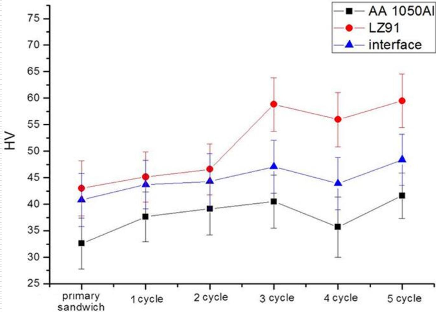
Variation of microhardness of Al layer, interface and LZ91 layer with increasing numbers of the ARB cycle.
