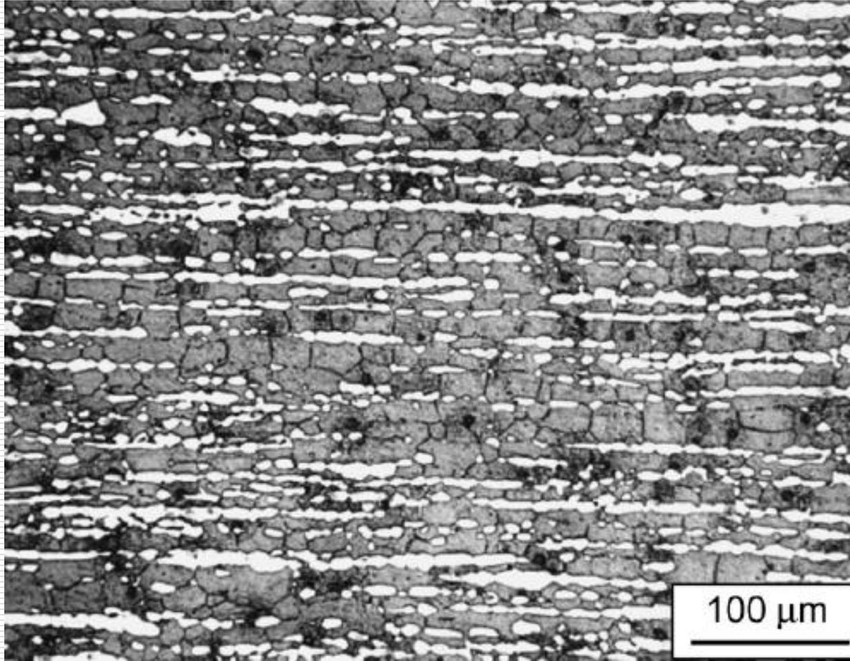
Optical microstructure of the starting LZ91(9wt.% Li-1wt.% Zn) sheet. Dual phases of LZ91 with  $\alpha$ -Mg and  $\beta$ -Li. The grain sizes of  $\alpha$ -Mg and  $\beta$ -Li were around 10-20 $\mu\text{m}$ .
