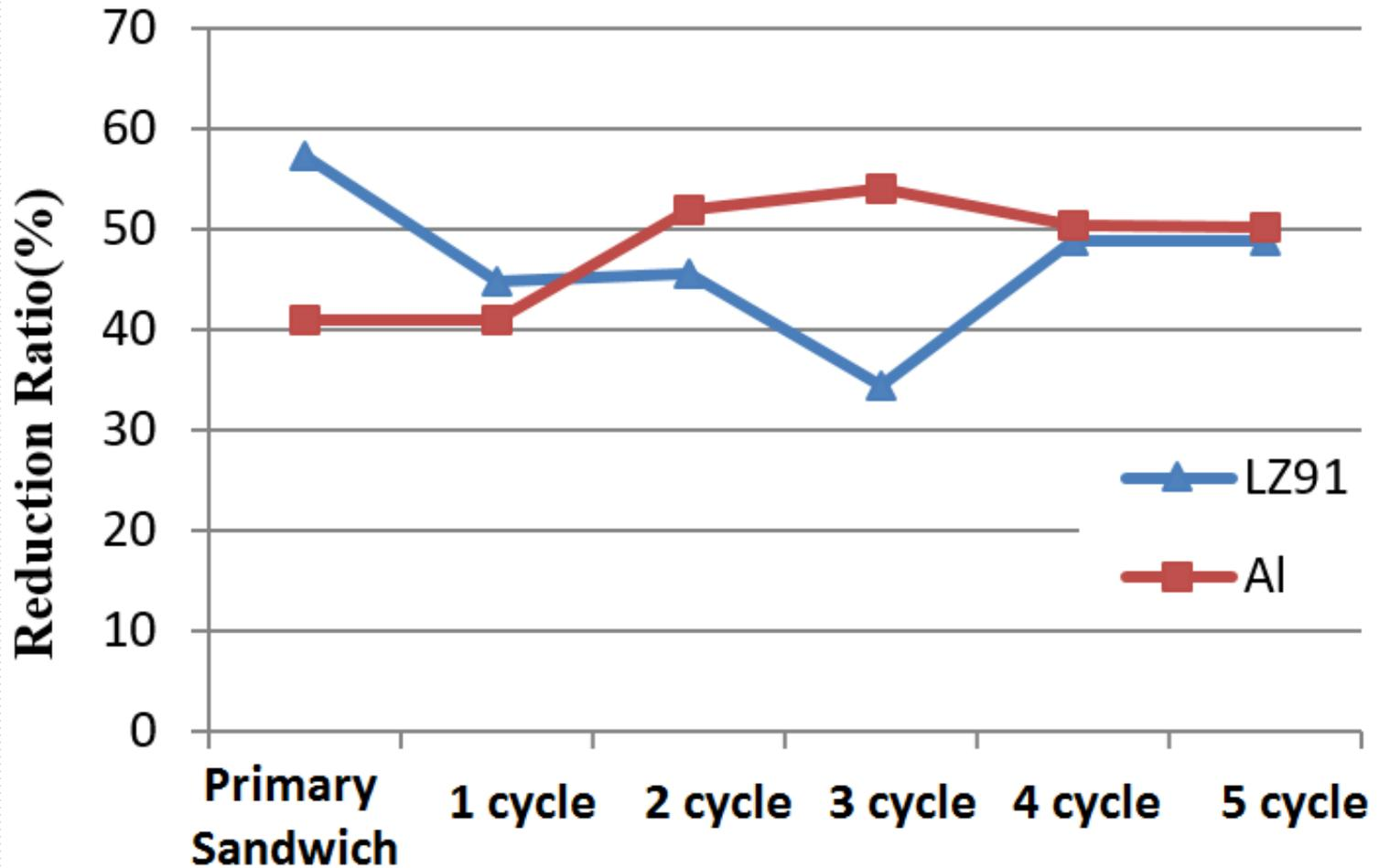
The thickness reduction ratio of the Al and LZ91 layers during each rolling process.
