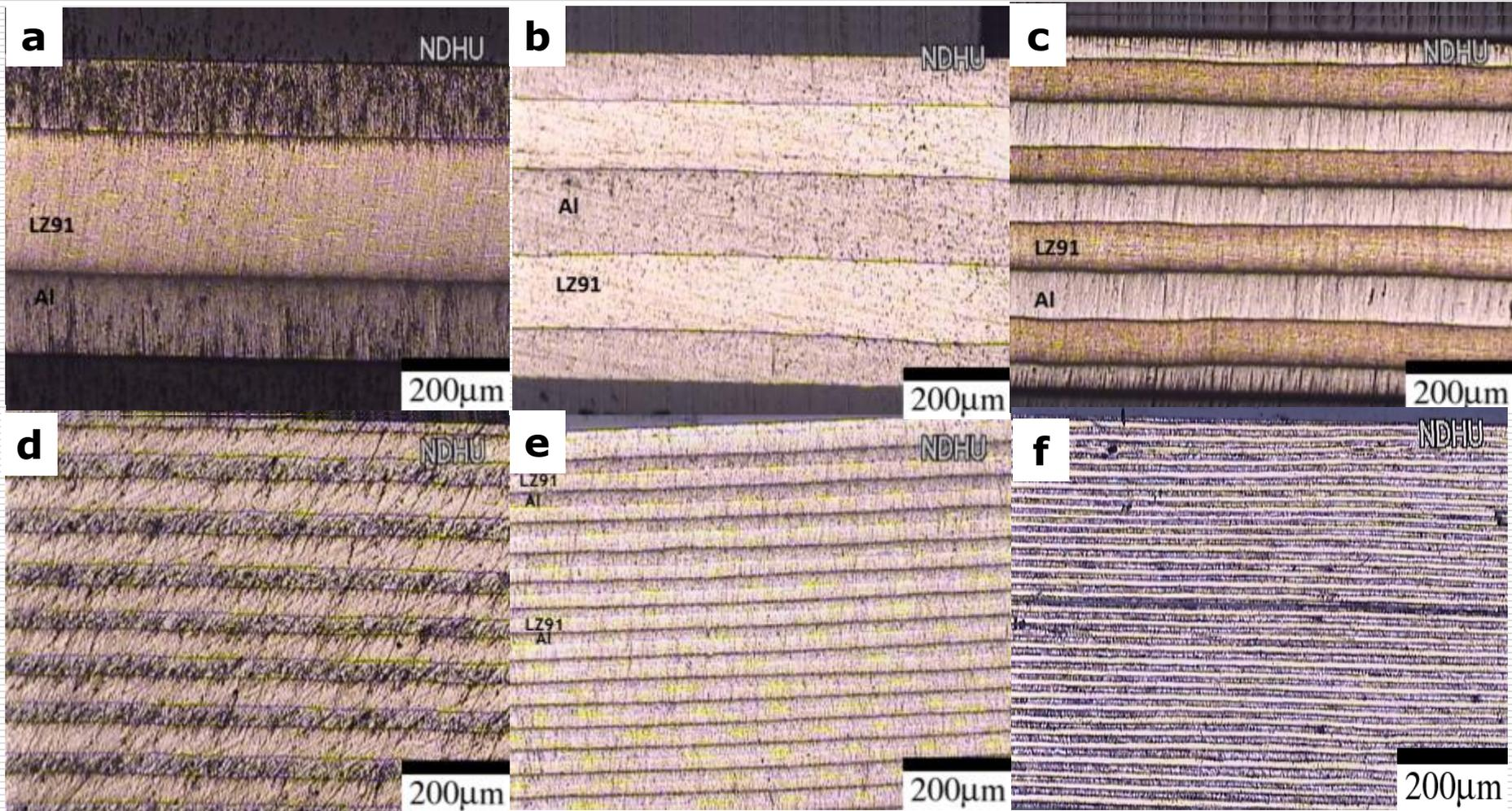
Optical micrographs of longitudinal cross-section of Al/LZ91/Al multilayered composites, (a) after primary sandwich preparation, (b) after 1 cycle, (c) after 2 cycles, (d) after 3 cycles, (e) after 4 cycles and (f) after 5 cycles.
