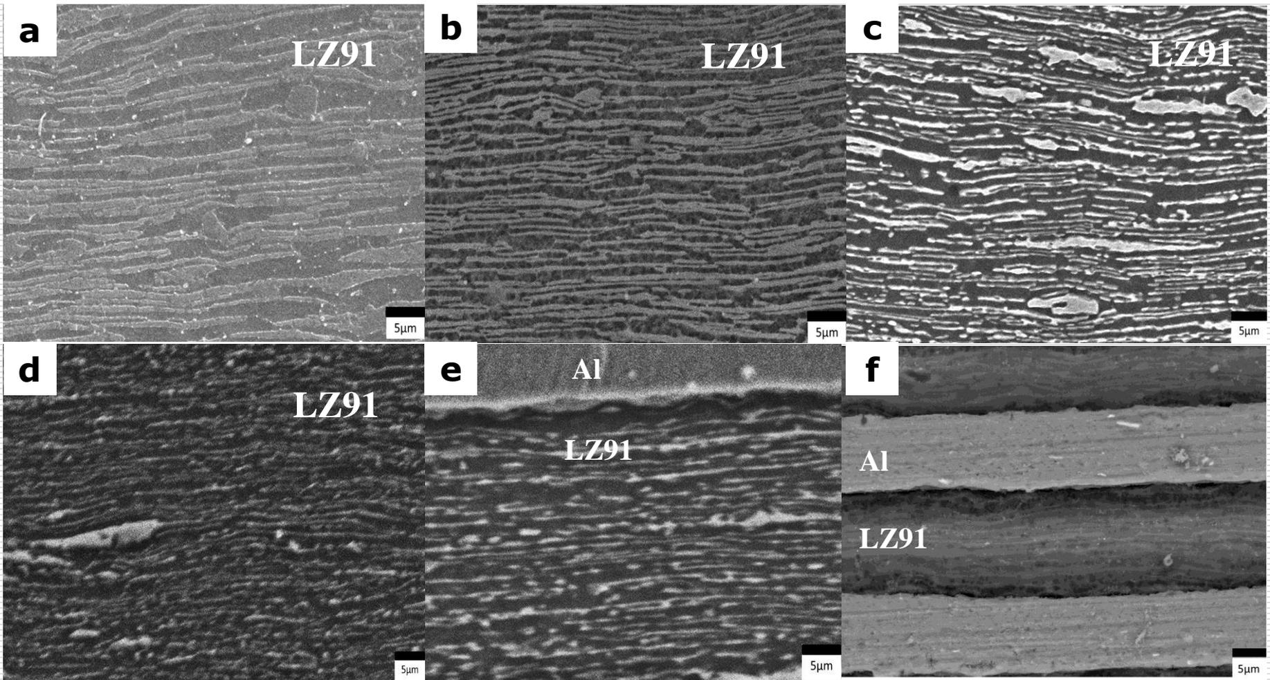
SEM microstructures of the LZ91 side in Al/LZ91/Al composite: (a) after primary sandwich preparation, (b) after 1 cycles, (c) after 2 cycles, (d) after 3 cycles, (e) after 4 cycles and (f) after 5 cycles.
