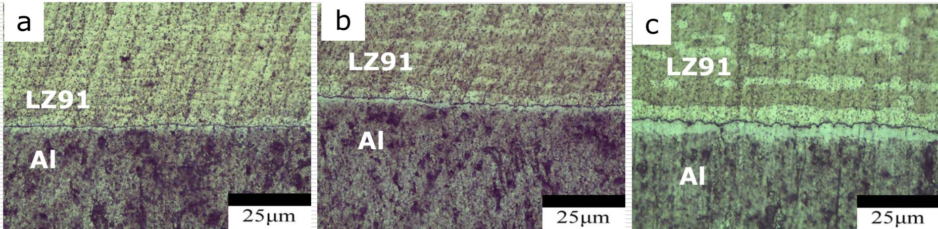
Cross-section optical micrographs of 1 cycle **ARBed Al/LZ91/Al** after annealing at (a) 473K, (b) 523K and (c) 573K.
