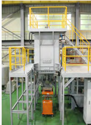
Thermal Reduction Furnace
