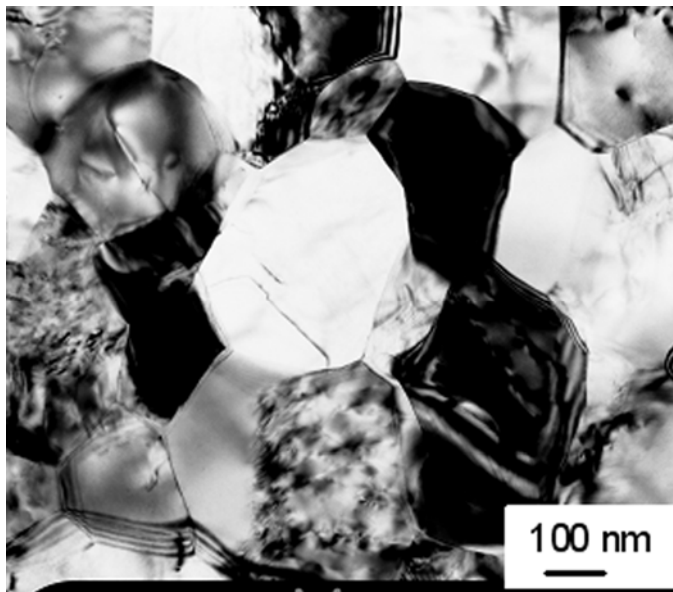
Grain structure of ECAP-modified titanium
